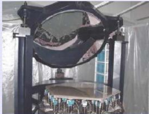
LAMOST segmented mirror & thin mirror active optics
