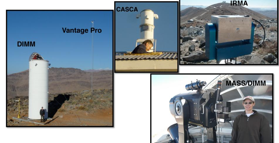
Figure 3: Photos of instrumentation in clockwise order: DIMM for seeing, Vantage Pro for meteorological data, CASCA for all sky images, IRMA for PWV and MASS-DIMM for turbulence profiling of the free atmosphere
