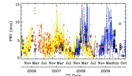
Figure 9: PWV as a function of time for a variety of sources at LCO and La Silla. The open boxes are MIKE spectra measured with the updated Brault method at LCO. The blue lines are IRMA data taken at LCO and calibrated with MIKE data. The red points are FEROS data from La Silla. The yellow lines are from the Erasmus model for the GOES-8 satellite (corrected by subtracting 2.5 mm as the median difference between the GOES-8 and FEROS medians at La Silla).
