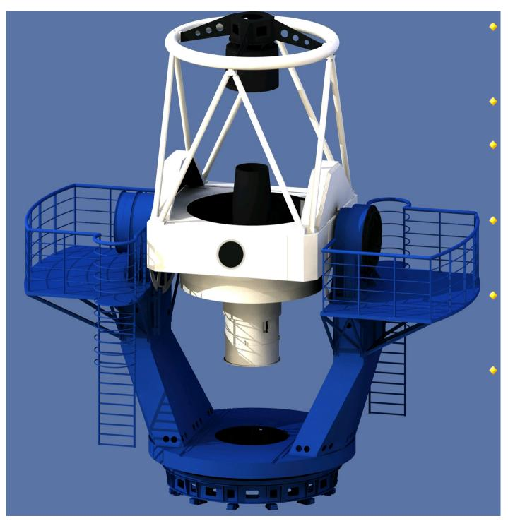
D 2.5m, RC f/8, M1: f/2.2, rms 30nm d(EE80)=0.4" Alt-Az, DD, 3<sup>o</sup>/s, ε5<sup>''</sup>, 5 foci (N1-4, C, <2min) C,N1: derotators, FOV 40' (WFC), AGU N2: optical prism derotation, FOV 15' N3,4 : "student ports" (on-axis small instruments)
