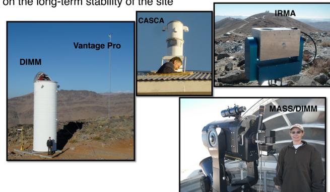
Figure 3: Photos of instrumentation in clockwise order: DIMM for seeing, Vantage Pro for meteorological data, CASCA for all sky images, IRMA for PWV and MASS-DIMM for turbulence profiling of the free atmosphere
